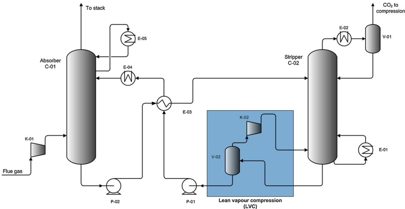
**Fig. 1.** Standard MEA plant with LVC. Main unit operations in LVC, which are flash vessel (V-02) and compressor (K-02), are highlighted. The rest of the equipment is included in a standard MEA process: flue gas blower (K-01), absorber (C-01), rich pump (P-02), lean pump (P-01), stripper (C-02), reboiler (E-01), condenser (E-03), lean-rich heat exchanger (E-04), cooler (E-04), and condenser drum (V-01).
