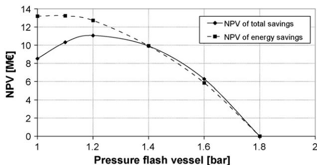
Fig. 2. NPV of total savings, and energy savings against LVC pressure. Case 1: design adapted to LVC operation.
