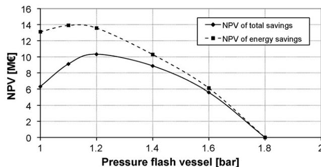
Fig. 3. NPV of total savings, and energy savings against LVC pressure. Case 2: retrofit of LVC to capture plant.
